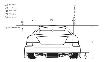
To assist competitors maintain consistent heights when using different wheels/ tyres, dimensions R and S will be measured with the chassis on a 15.0 mm block. Dimensions will be based on a 5 mm ground-clearance and will therefore be :- R = 122 mm, S = 45 mm.
