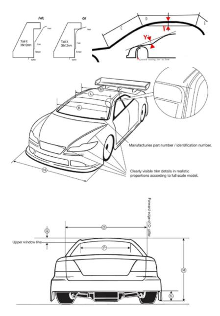
Maximum overall width (with body): 195 mm Maximum overall width (without body): 190 mm
